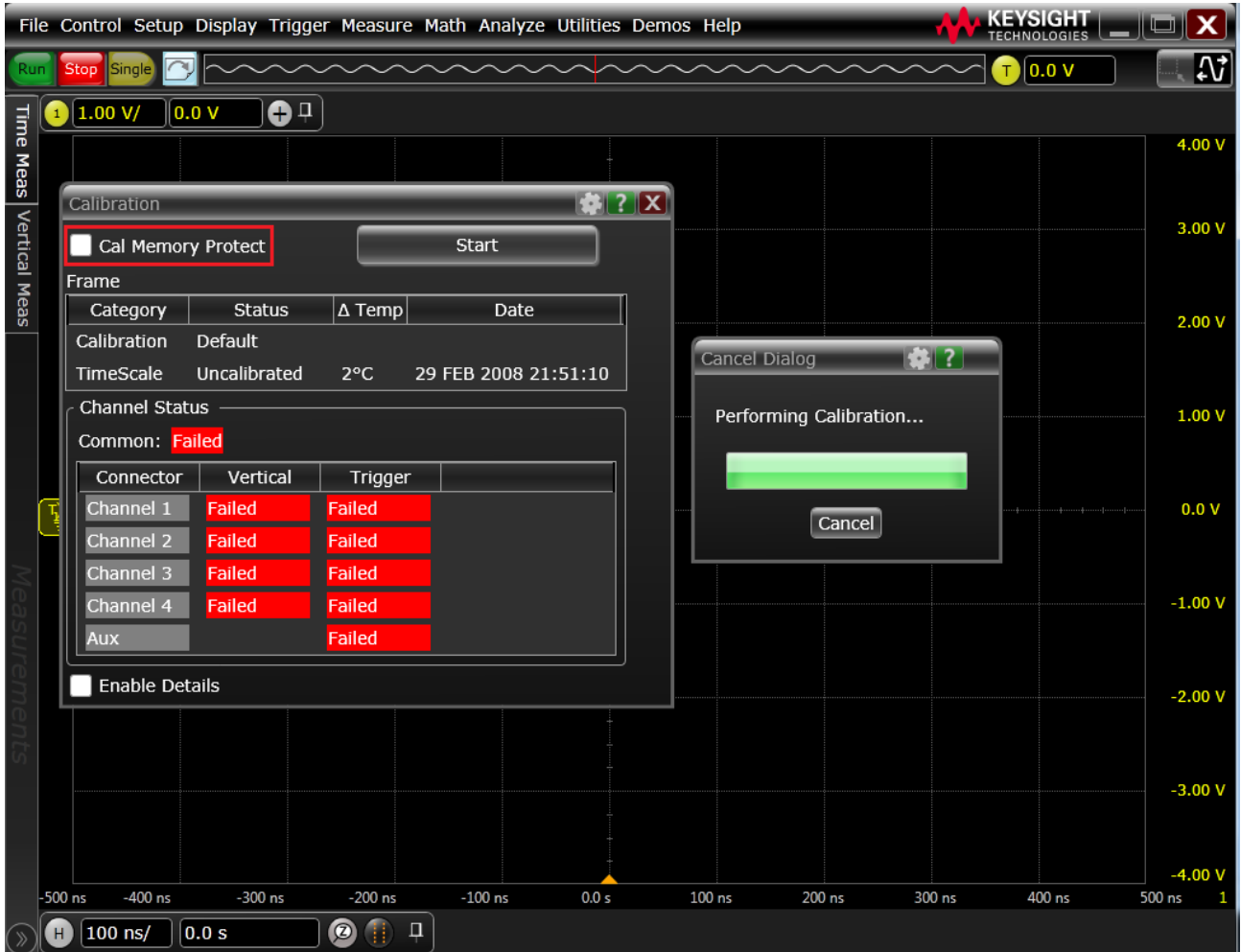
Figure 184 Clearing Cal Memory Protect and Starting Calibration
